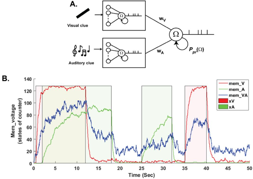
Fig. 6. Simulation of a simple hierarchical Bayesian network. (A) Schematic of the network (B) Evolution of membrane voltage of neurons activated by visual cue (red), auditory cue (green), and combined visual and auditory (blue) cues. Red and green rectangles show the presence of visual (xV) and auditory (xA) hidden variables, respectively, with some overlapping areas.
